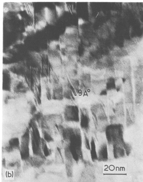
Figure 15 The mosaic structure of the V_2O_5 + 1 \text{ mol\% Fe}_2O_3 sample (a). (b) The same image much enlarged and (c) the electron diffraction pattern.
